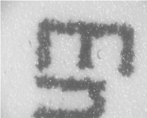
Figure 6. Printed pattern with the thermoplastic ink.
